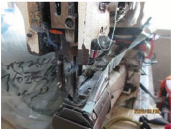
NC-No eyes' protective device equipped.JPG
